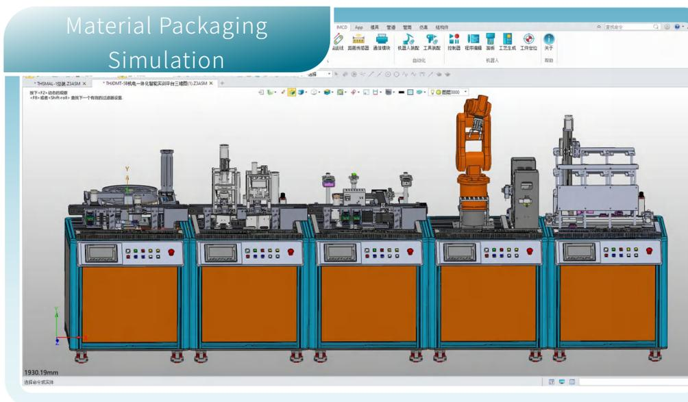
Material packaging simulation, including vibrating plates, multiple conveyor lines, robots, motor drives, material assembly, material transportation, and material warehousing
