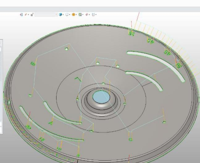
Uses processing solutions to quickly generate high-precision cutting trajectories, verify through physical processing simulation, import CL programs to convert into robot processing points, and optimize paths.
