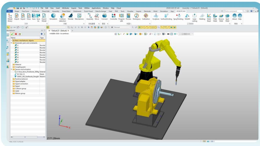
Uses CAD features for workpiece positioning, automatically generates multi-axis machining trajectories, and supports complex engraving applications for robots with 7+ axes.
